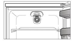
Air circulation fan will come on and go off from time to time while the fridge door is shut after use to circulate air in the fridge. This forced air circulation will improve the temperature maintenance in the fridge compartment. Do not block, obstruct or tamper with the fan or fan guard. Keep the fan guard free from food items and other objects.
